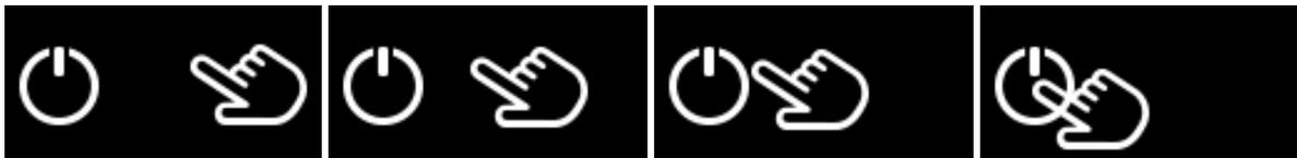
Hold the power touch button for a few seconds. The progress bar on the OLED screen shows the remaining time.
